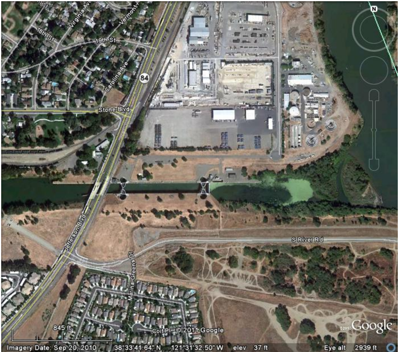
Google Earth aerial of the Sacramento River lock Note serious siltation between the east end of the lock and the river. Lock appears to be closed.
