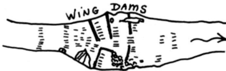
A set of Wing Dams at Eppes Falls on the Appomattox, as drawn by John Couty in 1834.
