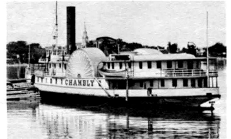
"Side-wheeler" of the type in use on the Chamblay Canal in the late 1800's.
