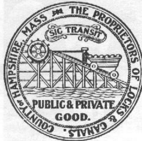
Seal of the Proprietors of Locks and Canals, showing the contrivance first used at South Hadley for passing boats.
