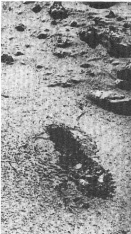
"Groundbreaking" for the Rocky Flats Canal (Valles Vikingis) - the first modern canal on Mars! Actually, what we see here is a trench dug on July 28, 1976 by the Viking 1 surface-sampler (lower portion of photo). Lumpy piles of material in the trench were left by the sampler backhoe. Area around the trench has ripple marks produced by the Martian wind. (NASA Photo.)
