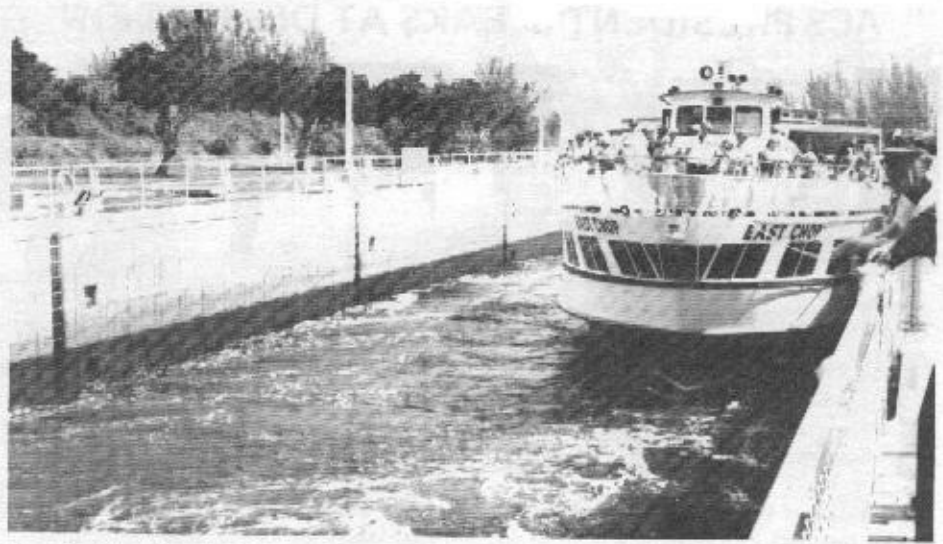
A cruise boat in the St. Lucie Lock, headed for Lake Okeechobee (looking east). This lock is 250 feet long, by 45 feet wide. The old, original lock is to the left of this view.
