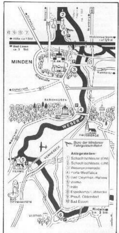
This map shows the unusual water "interchange" at Minden, West Germany, where Mittelland Canal crosses the Weser River. The Minden Aqueduct is shown in the upper right sector.
