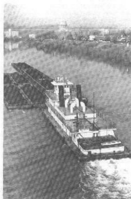
A typical, seven-barge tow on the Kanawha, with the capitol building at Charleston in the background. This configuration of barges has to be broken up at the locks. (Photo by Gerald Raffliff, West Virginia Chamber of Commerce.)
