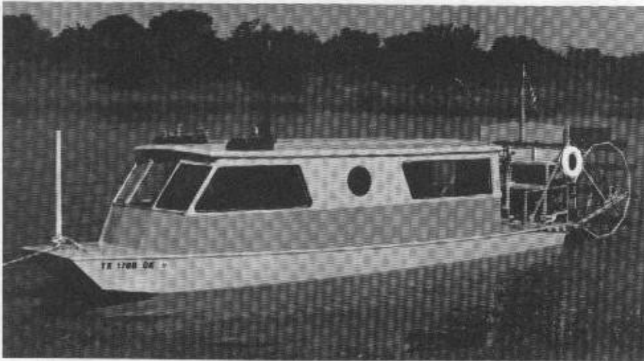
Fred D. Fleming, ACS member of San Antonio, Texas, sends this picture of his "stern-wheel powered canal boat, Icie Swiger" which he built himself. It is 35 feet long by 8 feet wide, all steel and "Trailerable." It is shown here on Canyon Lake near San Antonio, just the thing for shallow canals!
