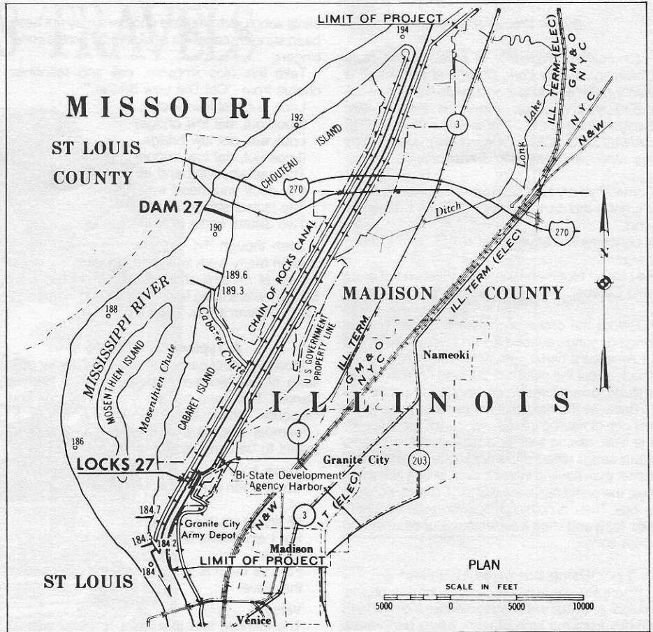
The Chain of Rocks Canal, built to by-pass a dangerous, swift-running reach of the Mississippi which contained many underwater ledges of rock. Completed in 1953, this short canal contains the southernmost lock (Lock No. 27) in the upper Mississippi lock-navigation system. (Map obtained from the Corps of Engineers by Walter Meseck.)
