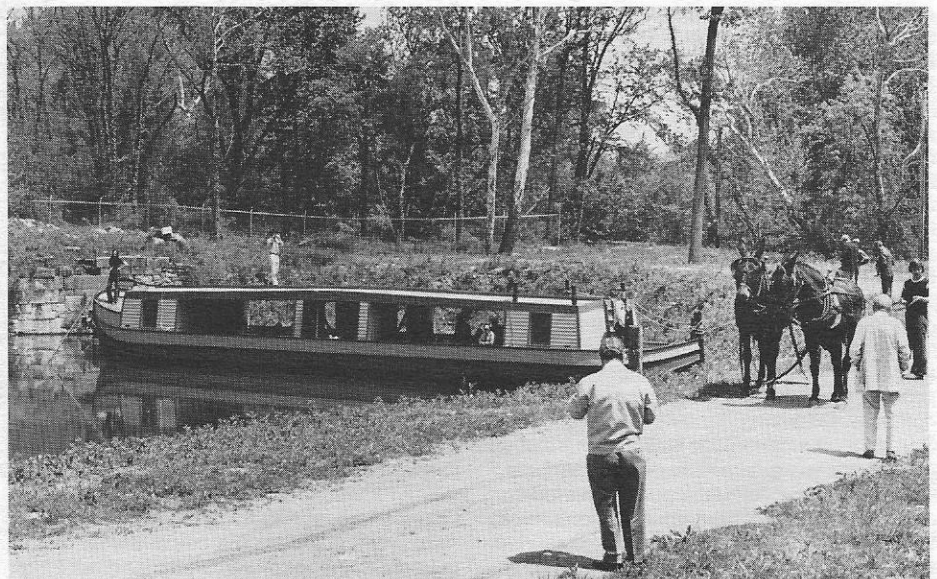
The "General Harrison", shown here on a re-watered section of the Miami and Erie Canal at Piqua is a replica of the old three-cabin Ohio freight boat. A roof has been added for the comfort of the 20th-Century passengers.
