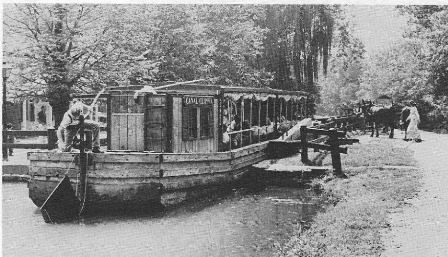
"The Canal Clipper" locks through the upper lock of the series of Locks on the C. & O. Canal at Great Falls, Maryland. The mule team, which tows the boat along several miles of the canal is visible at the right.
