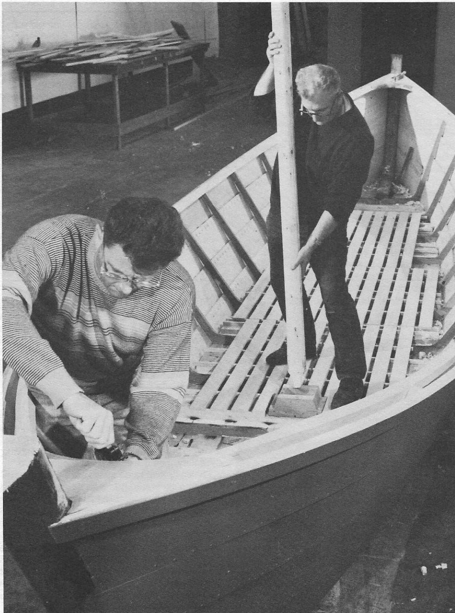
The "Discovery" — replica of an Eighteenth Century Batteau, such as used on the Mohawk River and early waterways west of Albany. Overall length: 30 feet, 4 inches. Maximum width at the gunwales: 7 feet, 3 inches. Carrying capacity: 1.5 tons.
