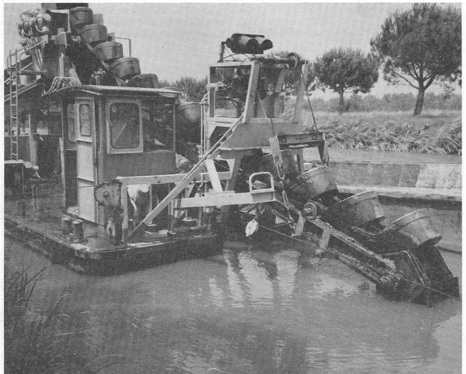
One of the dredges on the MIDI, which maintains the waterway at a five-foot depth. (Russell photo.)
