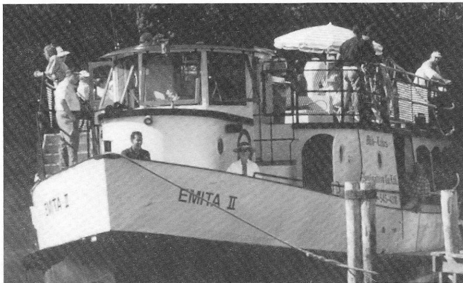
The Emita II, a former ferry boat, which has been reconstructed by the Mid Lakes Navigation Company to lower its superstructure to allow passage under the extremely low bridges of the western Erie Canal.
