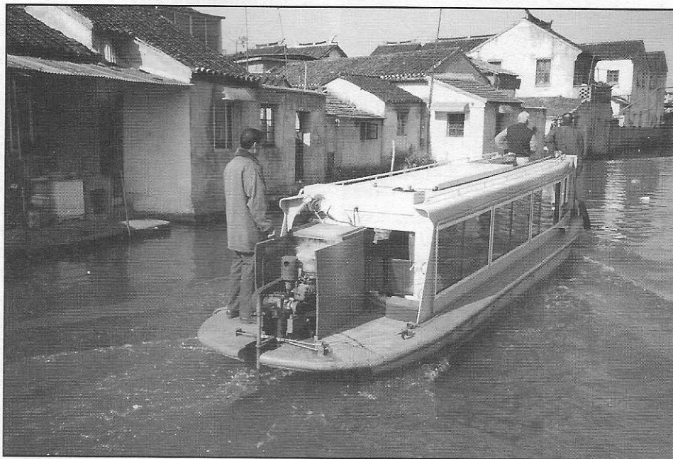
A commuter boat in Suchow, powered by a recycled diesel truck engine.
