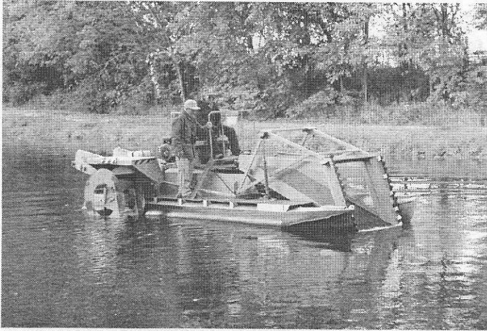
A good side view of "Queen Mary II" with the cutter head in its mid-point position.
