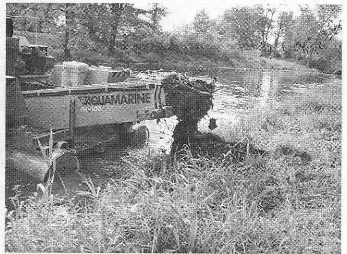
The harvester dumping its accumulated load of aquatic vegetation on the bank of the canal.
